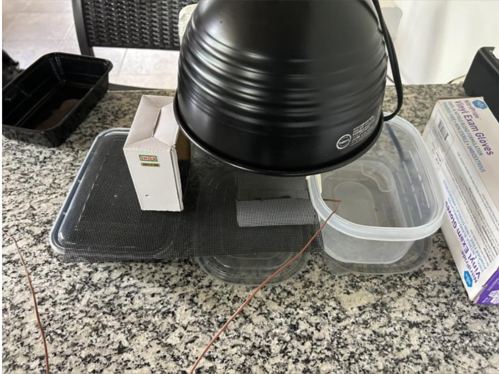
Figure 2: Testing chamber setup. A 100 W ceramic heat emitter bulb was used. A metal sheet was used to darken the heated chamber. A door was cut into the plastic tub and cardboard box to allow a frog to escape to the cooler but light plastic tub.
